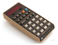
An improved version of the HP-25 featuring continuous memory, Programs and data were retained when the calculator was turned off, because the new low power CMOS memory was powered even in the "off" state. It was even possible to change the battery pack and retain the memory because of a capactor inside. Users expect continuous memory today but it was an impressive upgrade at the time. This was the first example of HP upgrading rather than replacing a calculation.
